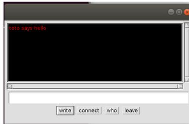
Above is the GUI of the Irc application. It has 4 buttons for which you have callbacks in the code, that you can adapt to implement communication between Irc instances. These buttons have the following meanings:
